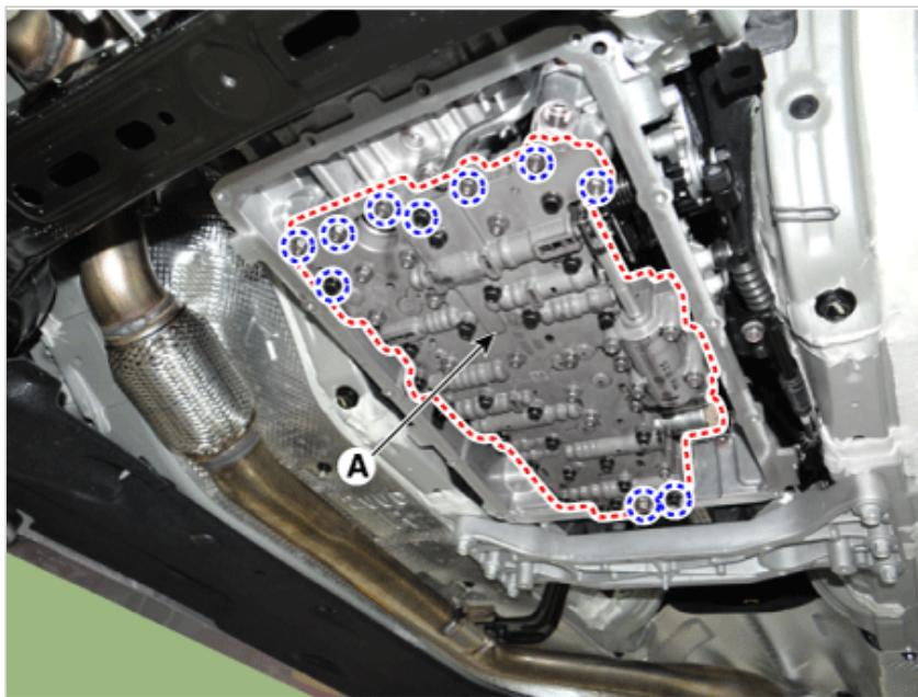
6. Remove the E-module (A) after loosening the bolts.
