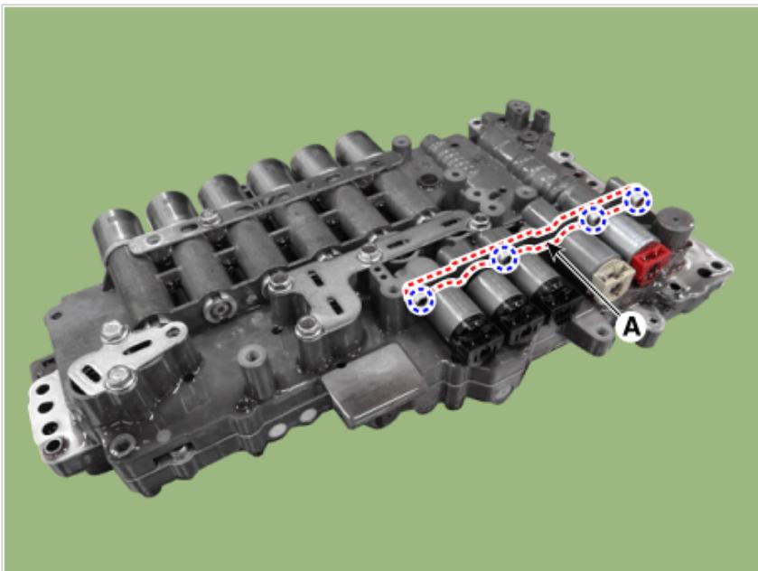
8. Remove the P position solenoid valve (A).
